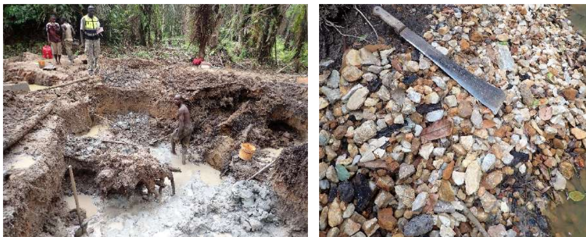
Photo 5 & 6: Extraction of alluvial gravels and waste heap at Glakpahyeepea creek
