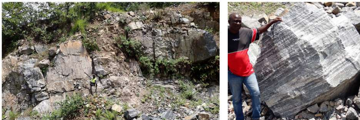
Jointing & fracturing of quartz diorite gneiss (striking 50° to NE) parallel to the Dube shear zone
