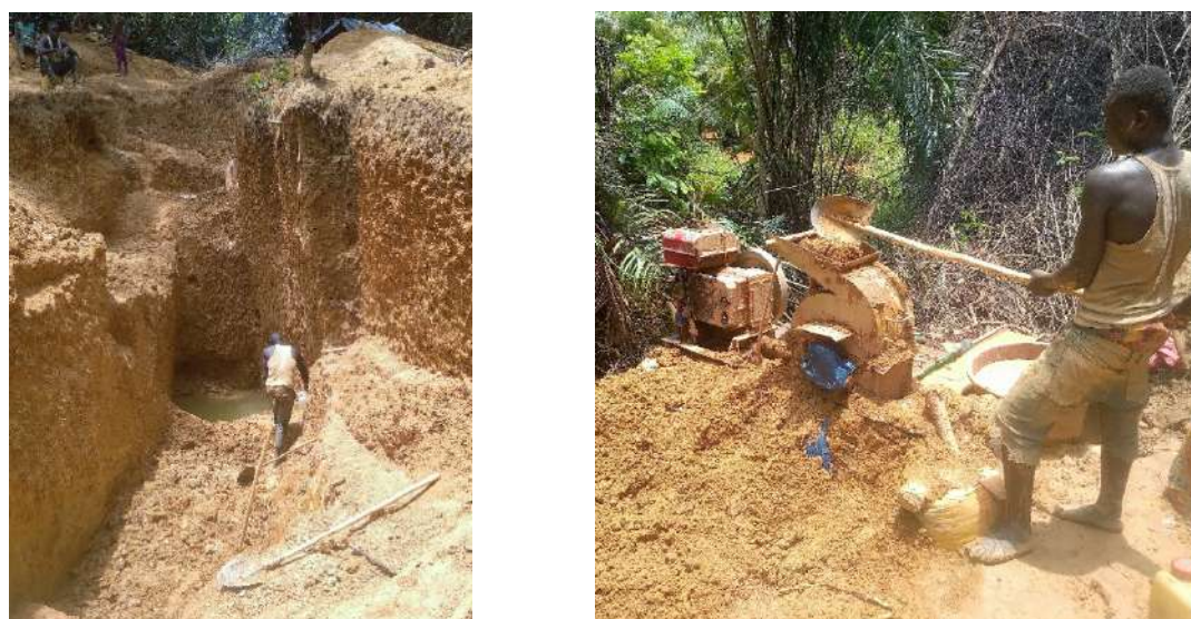
Photo 17: Excavation of mineralized weathered laterite & processing through Catacata
