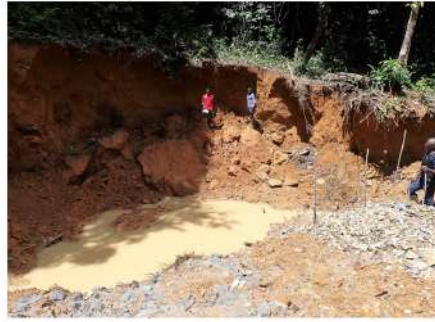
Spoil heap derived from washing of shallow surface lateritised saprolite
