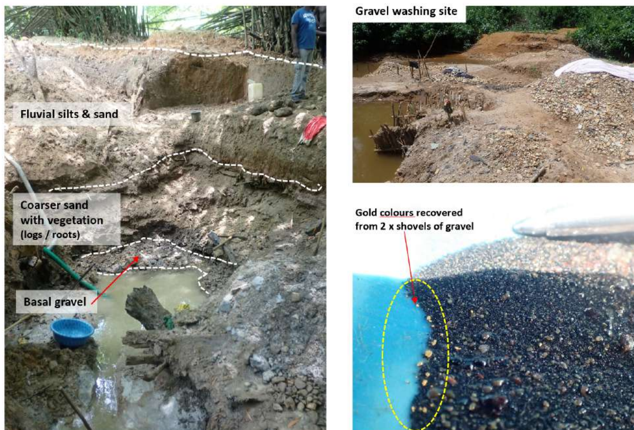
Photo 33: Locality 1, Site 3 mining of alluvial basal gravels at Domnemy
