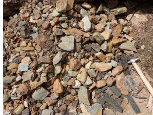
Photo 3 & 4. Carbonaceous metasediment sample, with schist, quartzite & banded iron-formation
