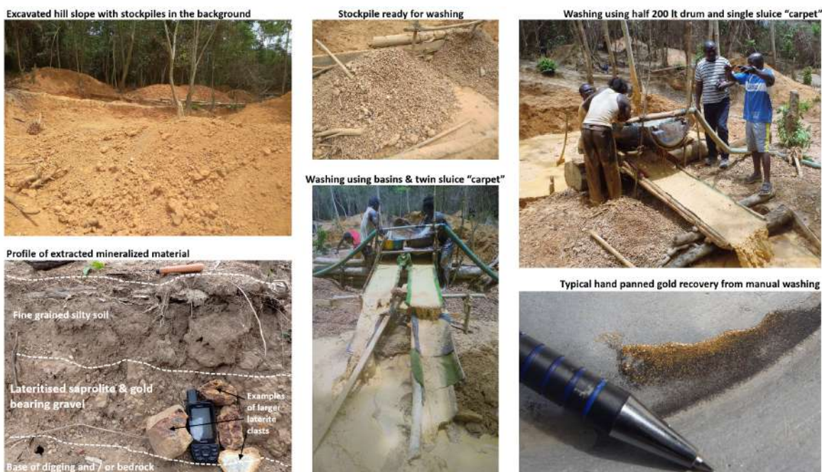
Photo 16: Extraction and washing of hill slope gold bearing saprolite and gravel
