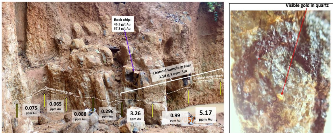
Figure 5: North face channel & rock chip sample results at the Ziatoyah discovery outcrop
