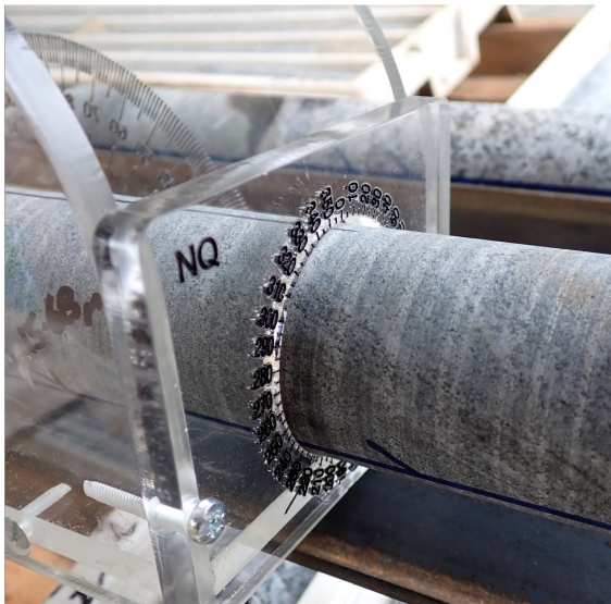
Structural measurements on core
